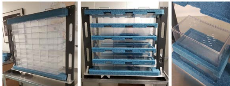
Fig 11. Housing array for mouse (panel A) and rat (panel B) irradiations in the 60 \times 60 \text{ cm}^2 beam. Exposure boxes, made of ~2mm thick polyethylene, stack together and are held in an array using a fabricated frame structure. (C)
