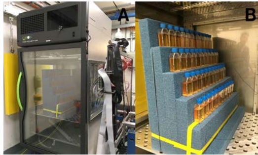
Fig 12. Modified incubator for use in beamline (A) with a holder that can accommodate up to fifteen T75 flasks in a 3 by 5 array or forty four T25 flasks (B).
