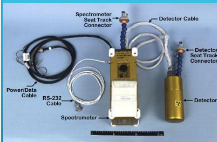
Figure 1: International Space Station Radiation Monitoring Instruments. From: http://srag-nt.jsc.nasa.gov/SpaceRadiation/How/How.cfm#Equipment
