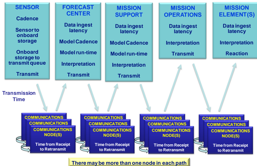
Figure 5: A comprehensive communications architecture considers much more than up-link and down-link antennas (From Turner, 2010).
