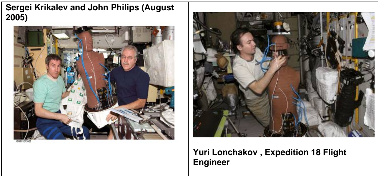
Fig.7: Removal of the Poncho (left) and removal of the detectors from inside the phantom by lifting up the MATROSHKA slices
