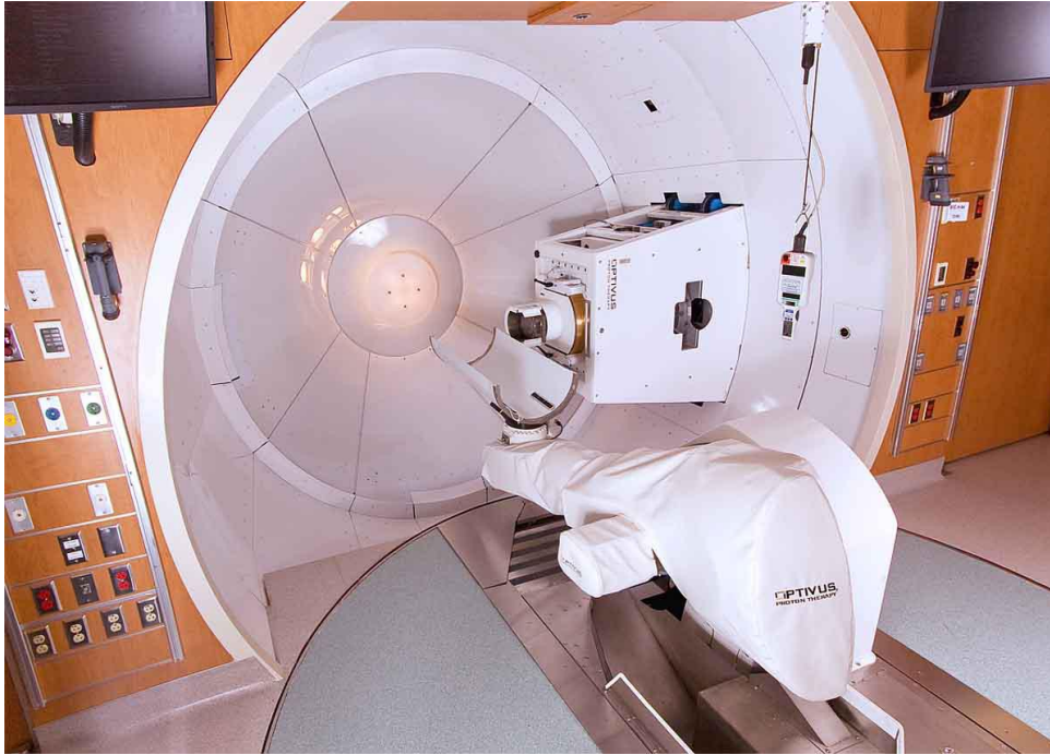
Robotic positioner in one of the gantry rooms at the James M. Slater, M.D., Proton Treatment and Research Center.
